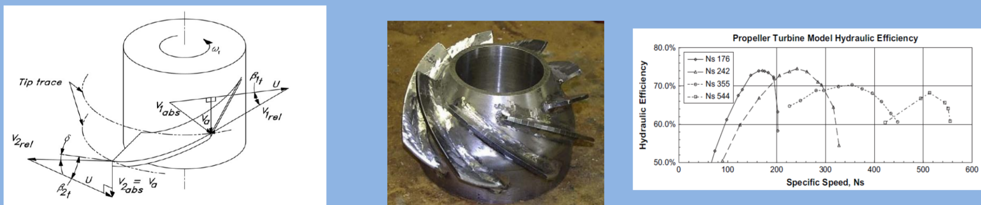
Fig.2 Conventional Axial and mixed flow runner prototype models and performance comparison[2]
