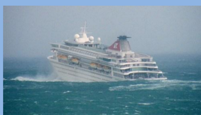
Added resistance is mainly due to heaving and pitching
