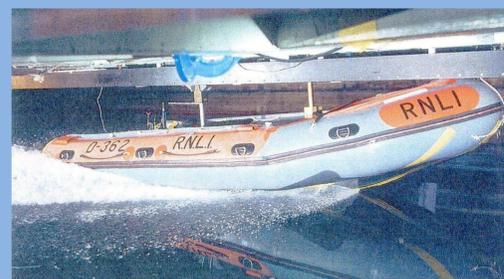
Left: shows the spray produced by the IB1, CPC have a chine to cleanly separate the spray but the spray on the IB1 adheres to the sponson [Dand (2003)]
