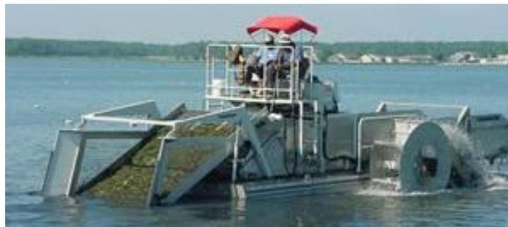
**Figure 28:** Illustration of Algae Harvesting Process
