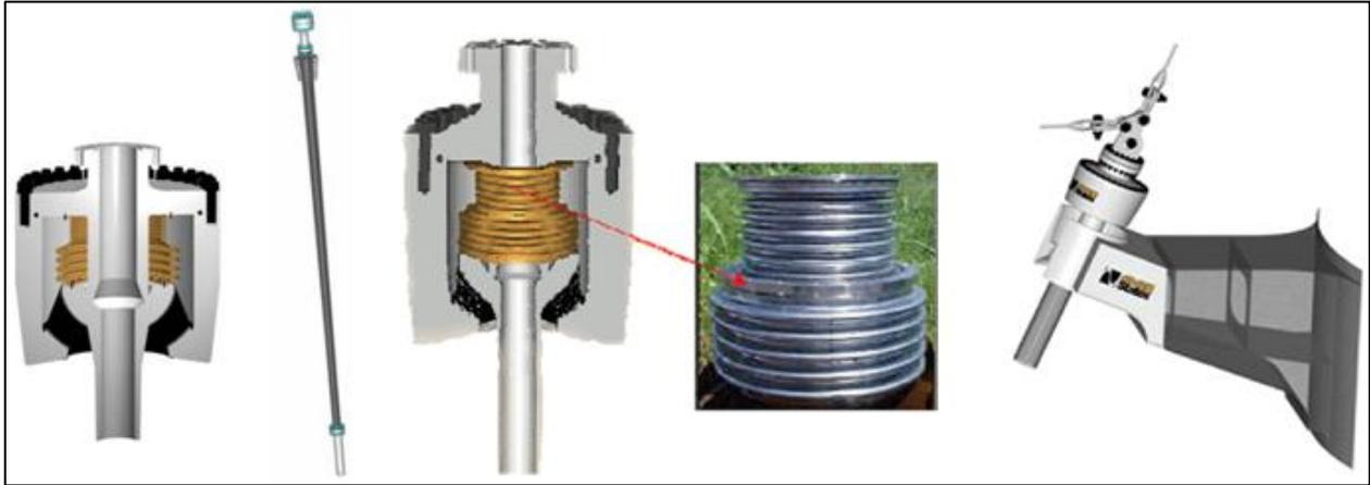
**Figure 71: SCR Hang-Off Systems: Flex Joint and Stress Joint**
