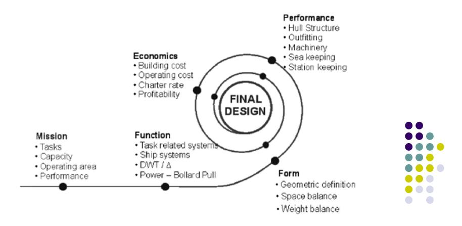
Figure 3: System Based Ship Design Spiral (Adapted From Erikstad and Levander, 2012)
