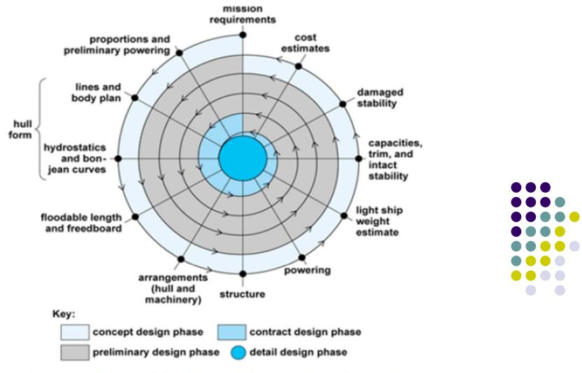
Figure 3: Example of a Typical Ship Design Spiral (Lamb 2003)
