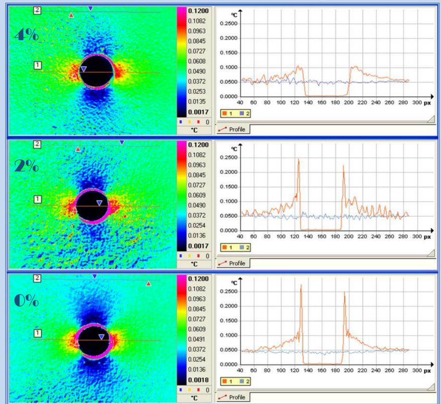
A variation in thermoelastic response from the areas around the cold expanded holes can be seen for each level of expansion (0%, 2%, 4%).
