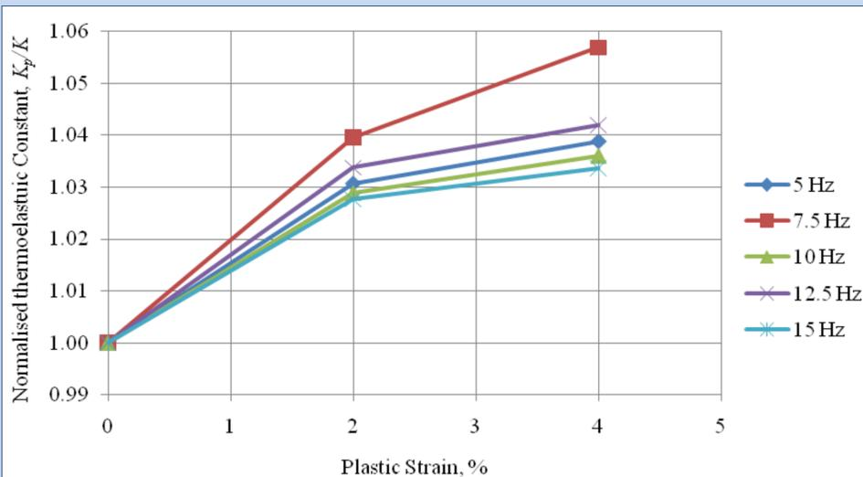
The thermoelastic constant for stainless steel 316L can be seen to increase with increasing plastic strain. Different loading frequencies have been used to evaluate the effect of the surface coating on the thermoelastic response.
