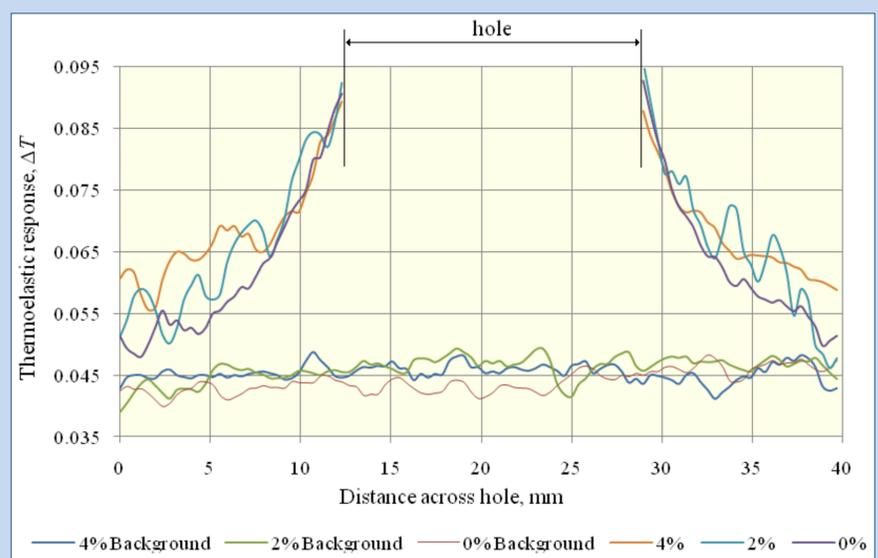
The differences in thermoelastic response could be due to the mean stress effect (which is prominent in aluminium) or plastic deformation due to hole expansion. Further work will investigate the origin of the changes. Noise can be seen around the holes and steps will be taken to minimise this, while maximising the thermoelastic signal and performing a point by point comparison of the data.
