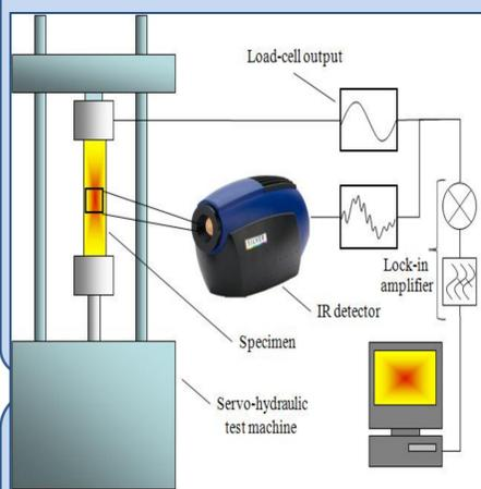
At present three approaches have been investigated for residual stress measurement using TSA. Two utilise the effect of mean stress on the thermoelastic response, the third investigates the effect of plastic deformation. This work examines the change in thermoelastic constant,  $K$ , due to plastic deformation
