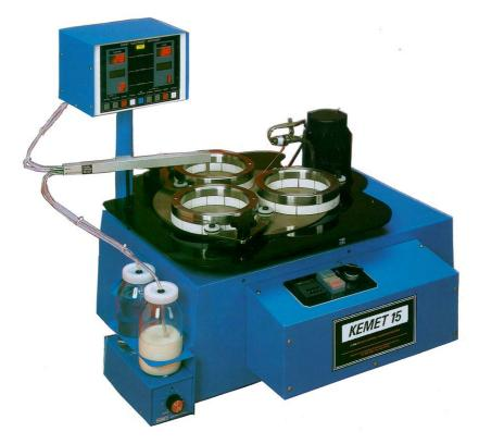
The Kemet 15 is a bench mounted Lapping Machine of rigid metal construction with a Work Table, adjustable for height. It incorporates a digital Process Timer and a fully automatic Liquid Diamond Dispensing System.
