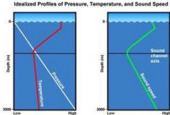
Figure 49: Idealized profiles of pressure, temperature and sound speed (COMET)
