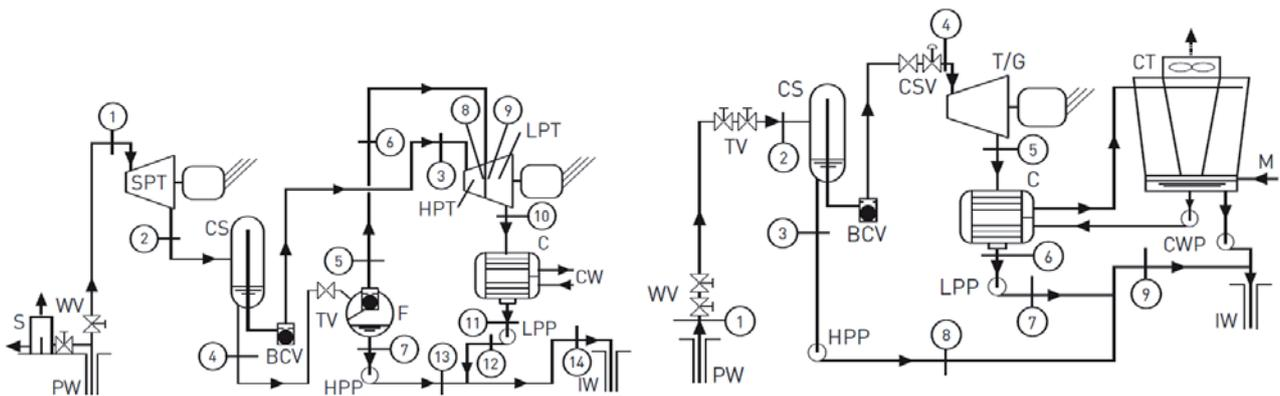
**Figure 3-5:** Plants for Supercritical Separated Hydrothermal Fluids; Triple-Expansion (left), and Single-Expansion for Ultra-High Inlet Pressures (right)
