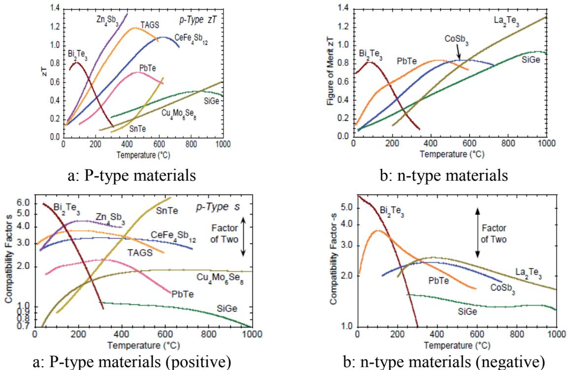
**Figure 3-11:** Compatibility Factors (*below*) and Figure of Merit (*above*) for Different (*a*) p-type and (*b*) n-type Semiconductors
