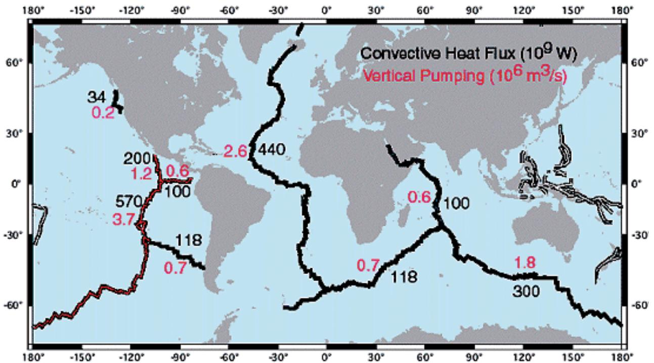
**Figure 2-6:** Heat Flux and Vertical Pumping along the Mid-Ocean Ridge (Source: NOAA)
