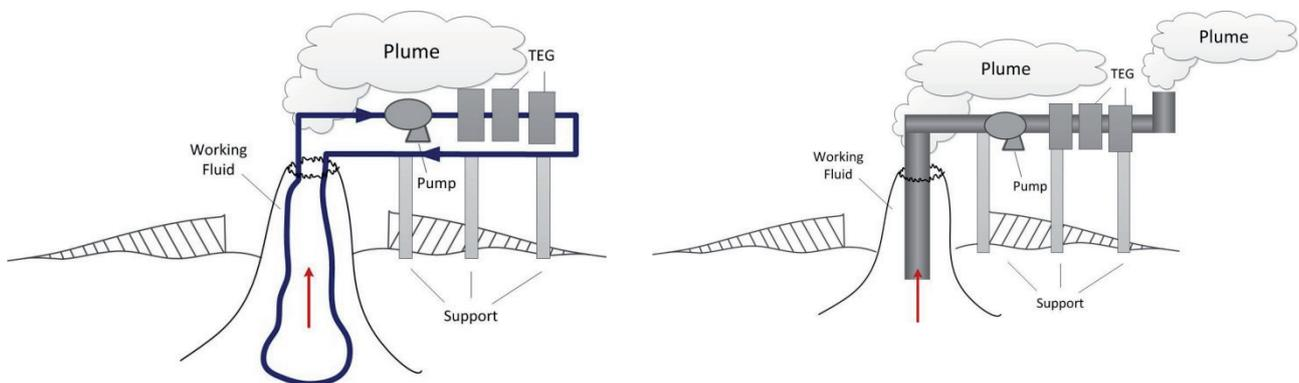
**Figure 4 -7:** Closed and Open Cycle Systems for Hydrothermal Energy Collection
