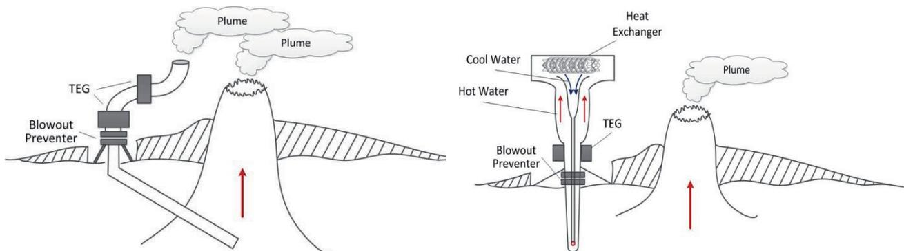
**Figure 4-4:** Drilling-Based Energy Collecting Systems
