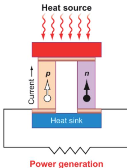
**Figure 3-6:** A Thermoelectric Couple to Achieve Power Generation
