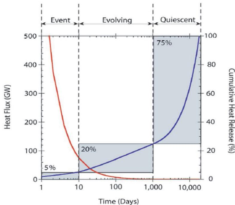
**Figure 2-3:** Graphical Representation of the Heat Flux (red curve) and Corresponding Cumulative Heat Release (blue curve) as a Function of Time at a Fast- or Medium-Spreading Ridge Crest (C. German & Lin 2004)
