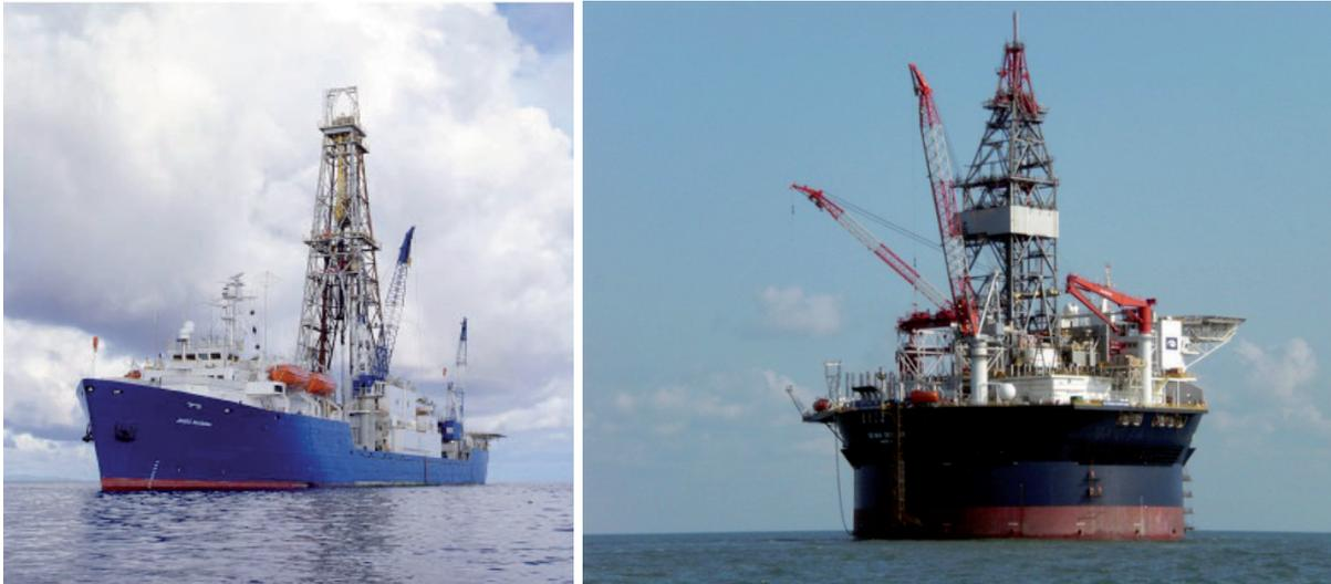
**Figure 4-3: JOIDES Resolution Vessel from the Ocean Drilling Program, and the SEVAN Driller from Petrobras.**
