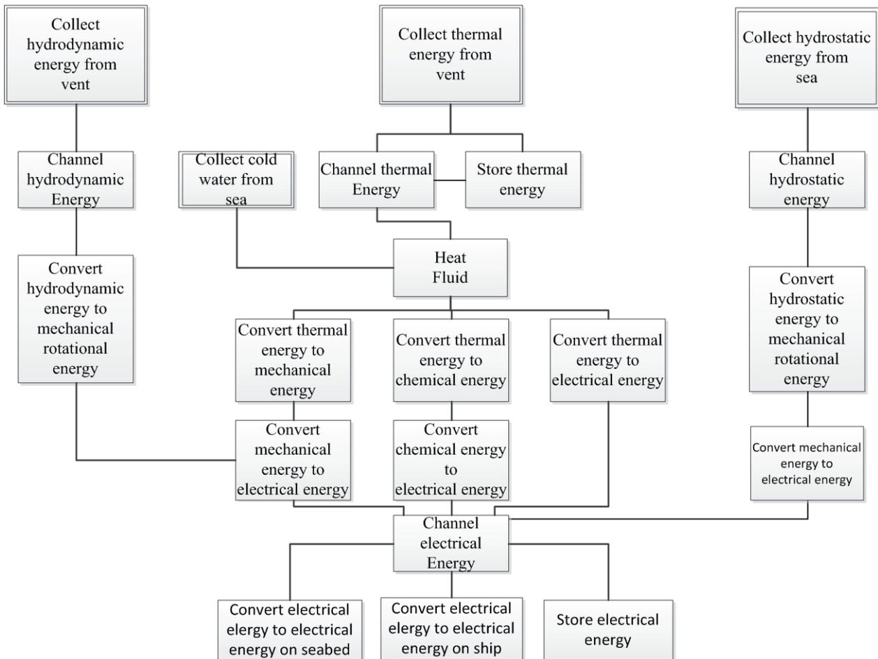
**Figure 3-2:** Functional Analysis of the Energy Conversion Sub-System
