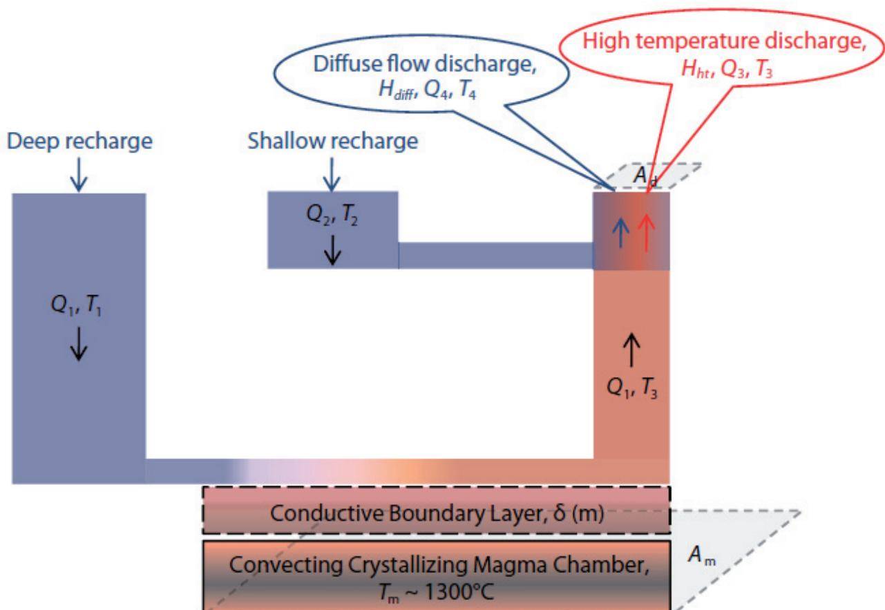
**Figure 3-10:** Schematic of a Cross Section of a Two-Limb, Single-Pass Hydrothermal Circulation Model for Understanding the Partitioning Between Focused and Diffuse Flows at the Vent-Field Scale (Bemis et al. 2012).
