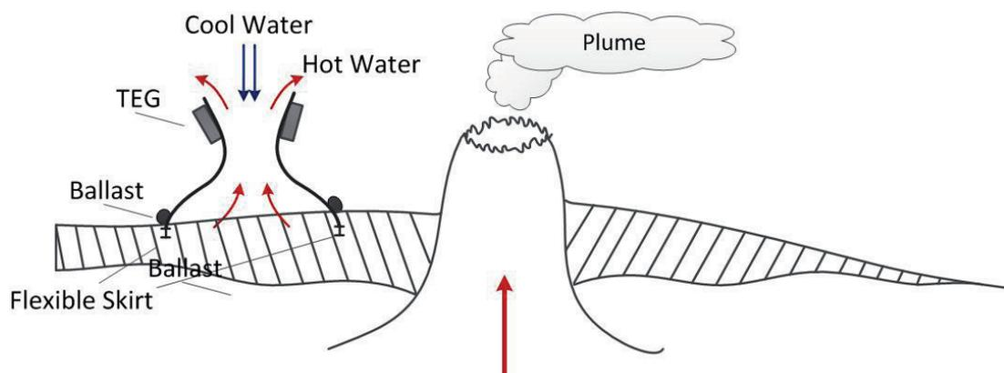
**Figure 4-5:** Hydrothermal Energy Collection by Venturi Unit
