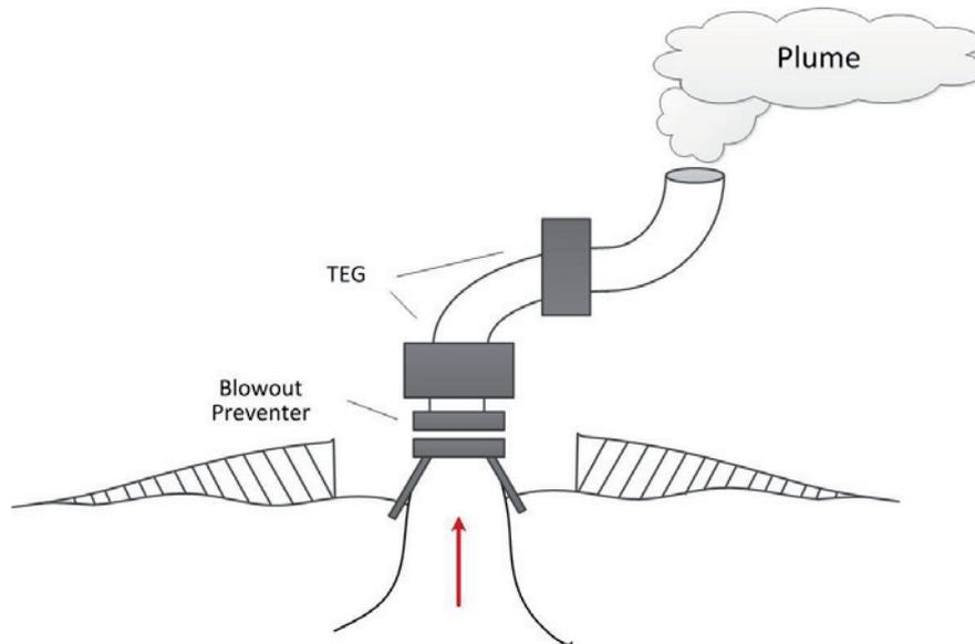
**Figure 4-6:** Energy Collection by Covering of the Hydrothermal Vent
