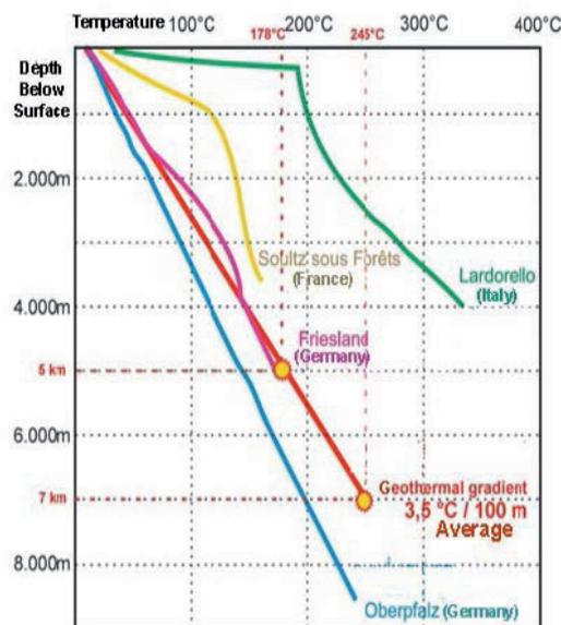
**Figure 1-5:** Earth's Crust Temperature Profile in Different Places
