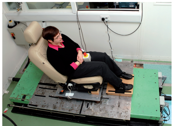
Horizontal vibrator: simulation of motion environments
