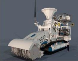
Bulk Cutter (BC) - puts material at high rates on area benched by Austiany Cubi
