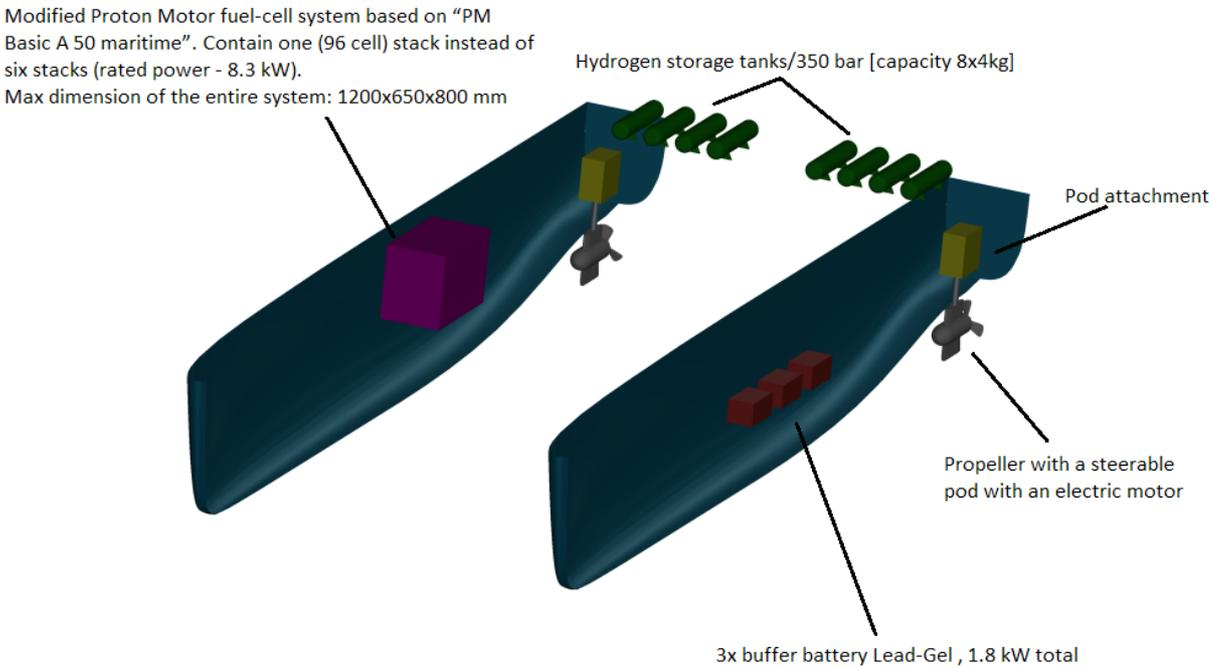
**Figure 59:** Technical data and general arrangement regarding the on-board installations.
