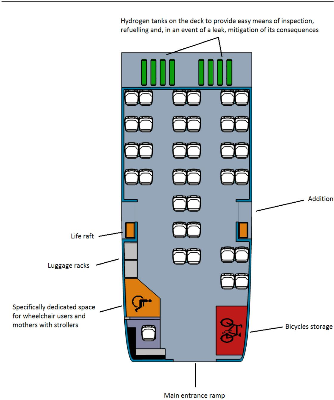
**Figure 60:** General interior arrangement plan.
