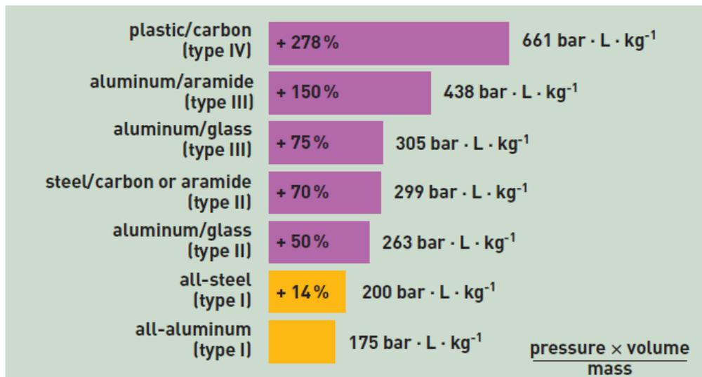
**Figure 63:** Comparative analysis of the performance factor (pressure · volume/mass) of various tank types (Isabelle Moysan CEA, 2004-2005).
