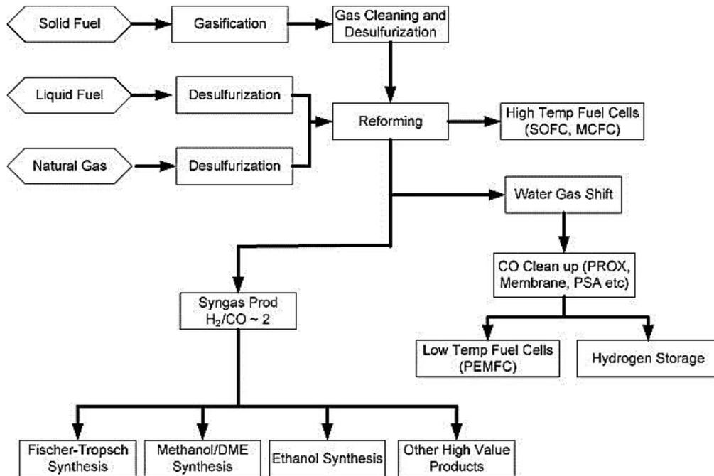
**Figure 31:** Hydrogen production through reforming of gaseous, liquid, and solid fuels (Holladay et al., 2009).
