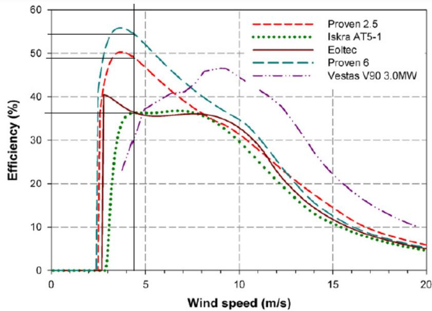
**Figure2:** Efficiencies of some commercially available micro-wind turbines as function of wind speed. Adapted from (Sissons et al., 2011).
