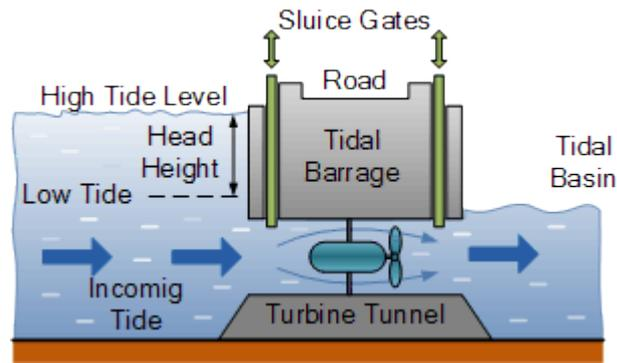
**Figure 21:** Tidal Barrage Flood Generation system<sup>11</sup>.
