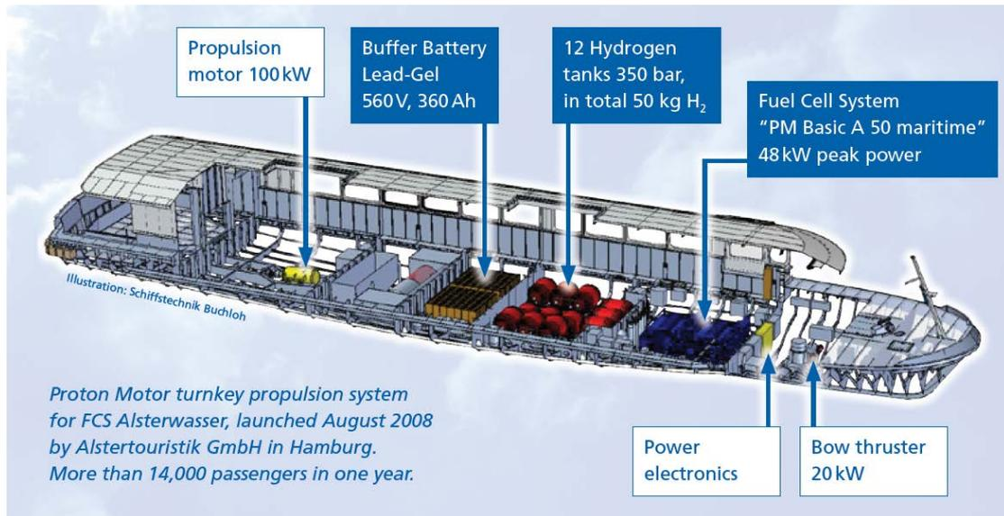
**Figure 53:** FCS Alsterwasser - general arrangement.
