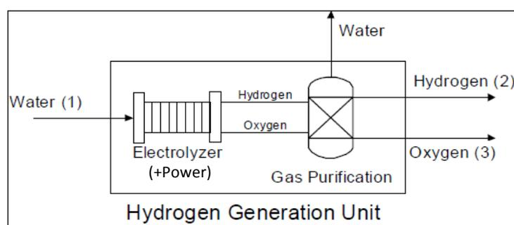
**Figure 33:** Sketch of hydrogen generator through electrolysis, adopted from (Laboratory, 2004).
