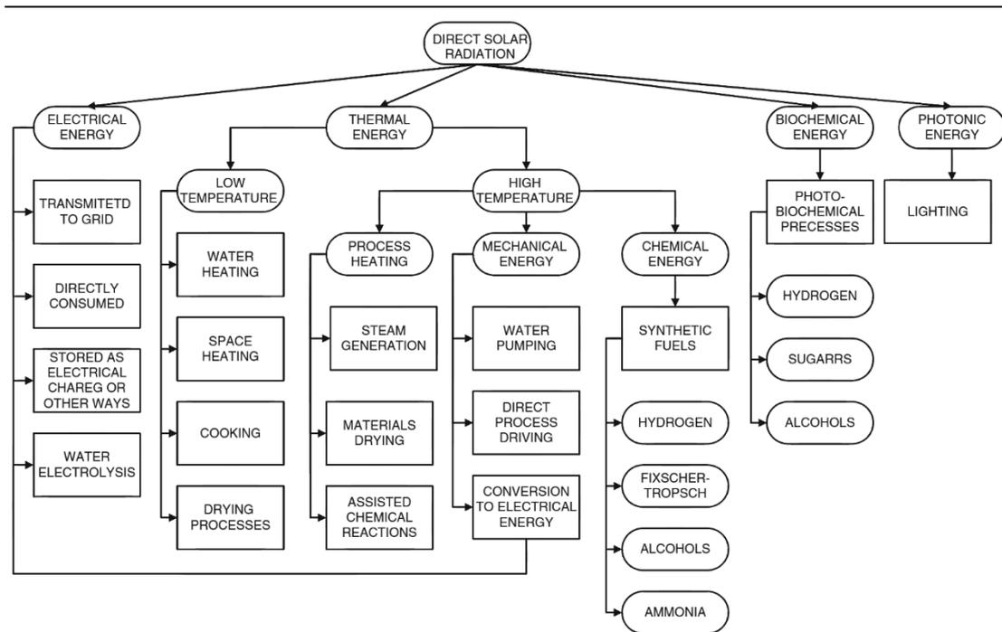
**Figure 12:** Conversion paths of direct solar radiation with engineered systems (Dinçer & Zamfirescu, 2011).
