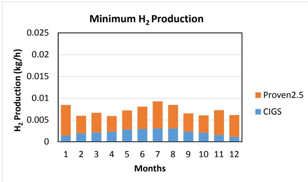
**Figure 68:** Monthly minimum H<sub>2</sub> production with the least productive components.
