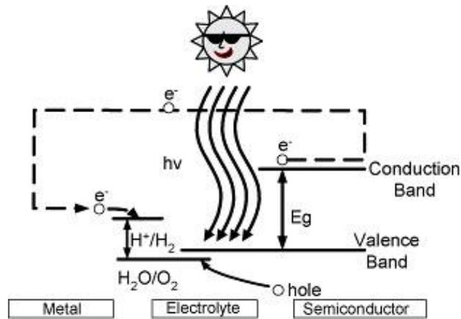
**Figure 34:** Energetic diagram of n-type semiconductor photo-electrochemical cells (Holladay et al., 2009).
