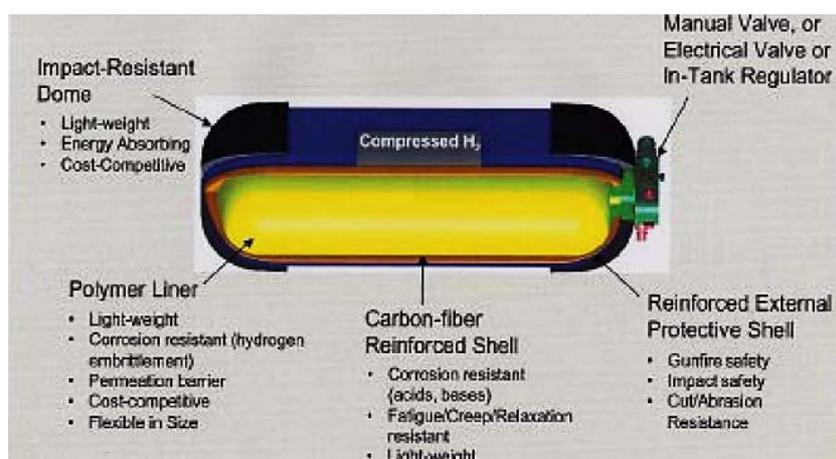
**Figure 35:** Schematic of a typical compressed H<sub>2</sub> gas composite tank (Riis et al., 2005).
