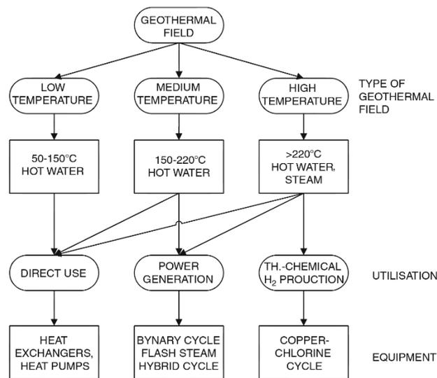
**Figure 22:** Classification of geothermal fields and utilization of geothermal energy (Dinçer & Zamfirescu, 2011).
