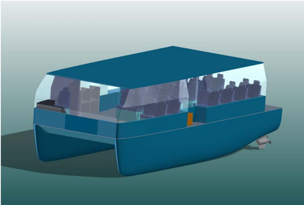
**Figure 58:** Hydrogen ferry designed for operation on Itchen River (Southampton).
