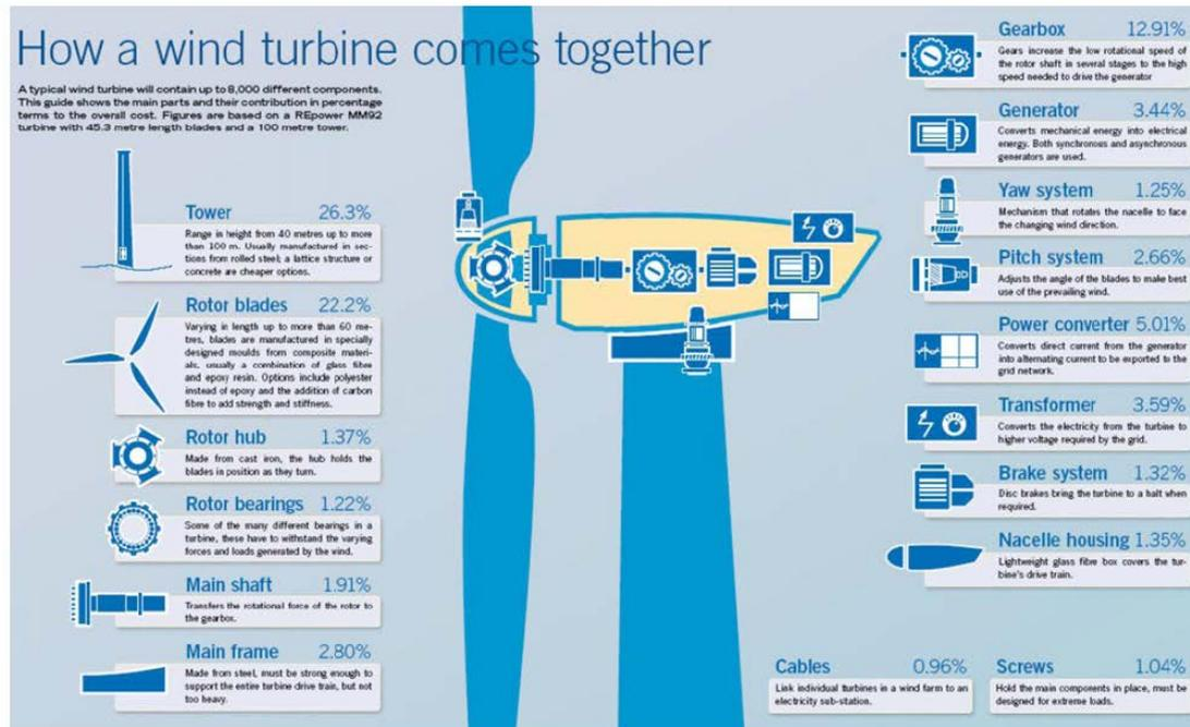
**Figure 15:** Main components of a wind turbine and their share of the overall cost (Shafiullah, M.T. Oo, Shawkat Ali, & Wolfs, 2013).
