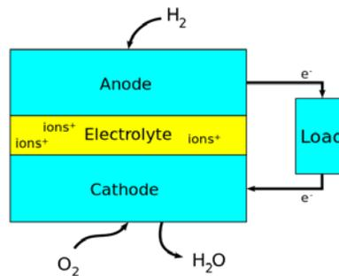
**Figure 37:** A block diagram of a fuel cell<sup>14</sup>.
