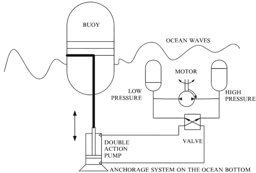
**Figure 19:** Principle of operation of buoy-type ocean wave energy conversion system (Dinçer & Zamfirescu, 2011).
