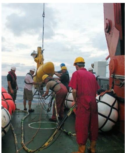
Tailbuoy and section of the 2.4 km 192 channel streamer used in the seismic reflection acquisition
