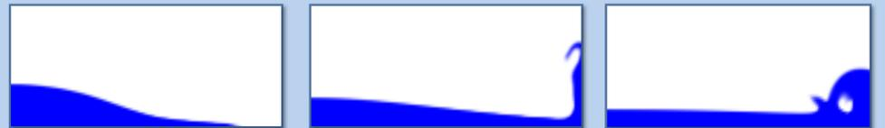
Pressure data is recorded and measurements compared to experimental data from the right hand wall 0.16m from the floor. Quantitative comparison is found for pressure everywhere but at the peaks due to the coarse mesh and the 1<sup>st</sup> order time discretisation scheme that was used in the CFD study.
