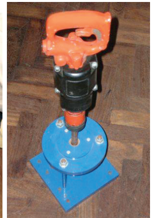
Laboratory measurement of vibration on vibratory tools
