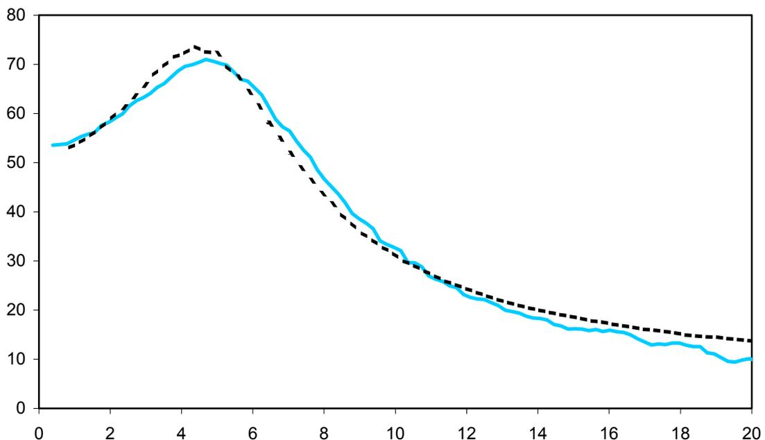
Measured apparent mass of anthropodynamic dummy measured using broadband random vibration at 1.0 ms<sup>-2</sup> r.m.s. compared to the Fairley and Griffin model (1989): Measured response, — modelled response, - - - - -
