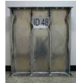
Mode V – stiffener-induced collapse by tripping
