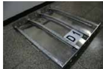
Mode III – stiffener-induced collapse by beam-column type collapse
